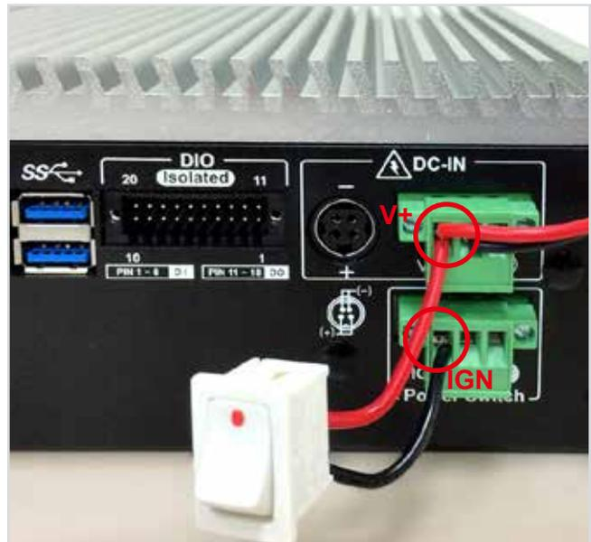
For testing purpose, you can refer to the picture above to simulate ignition signal input controlled by a latching switch.
