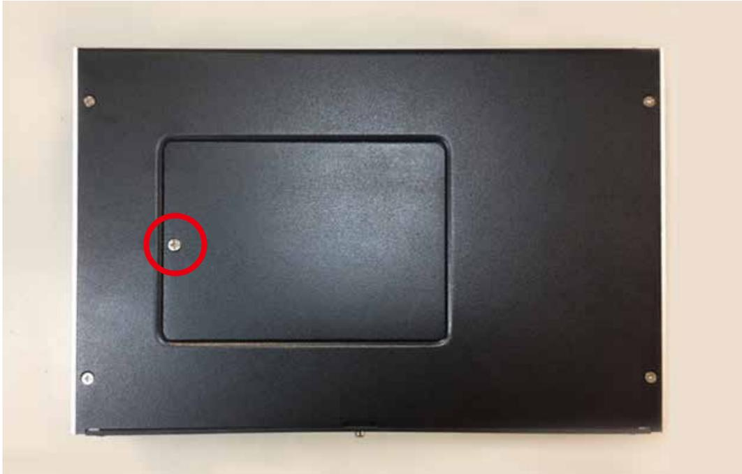
**Step 2** Install SSD/HDD with HDD bracket.
