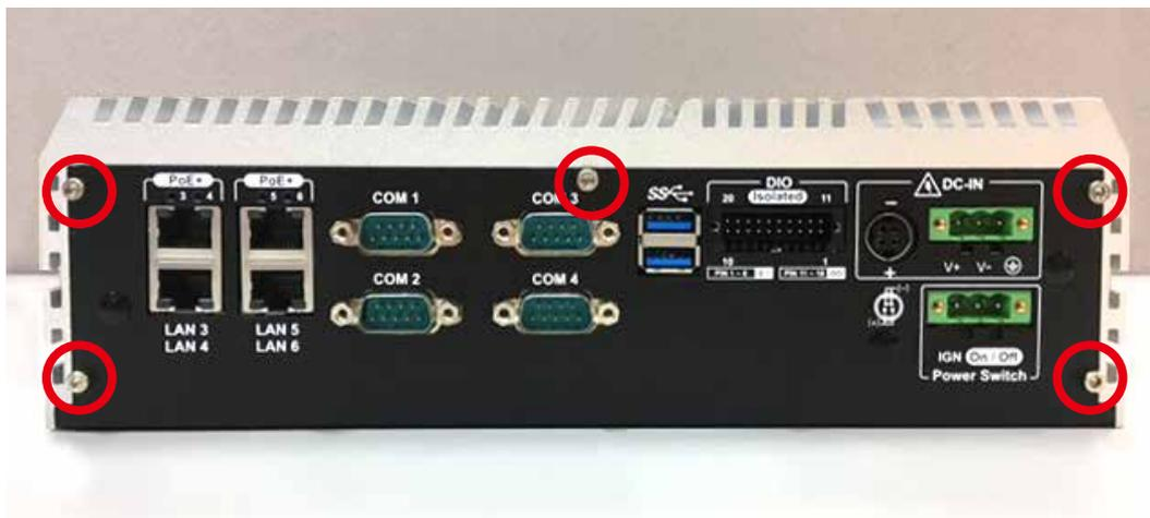
**Step 3** Remove bottom four F#6-32 screws.
