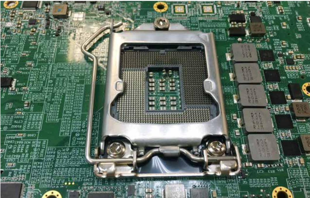
**Step 5** Installing CPU on the slot.
