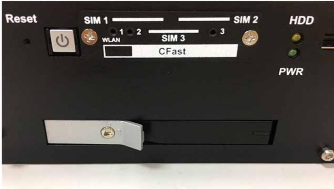
**Step 2** Use the trigger and open SSD/HDD tray.
