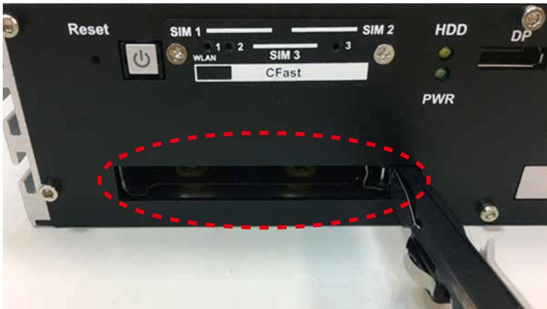
**Step 3** Installing 2.5" SSD/HDD into the tray.
