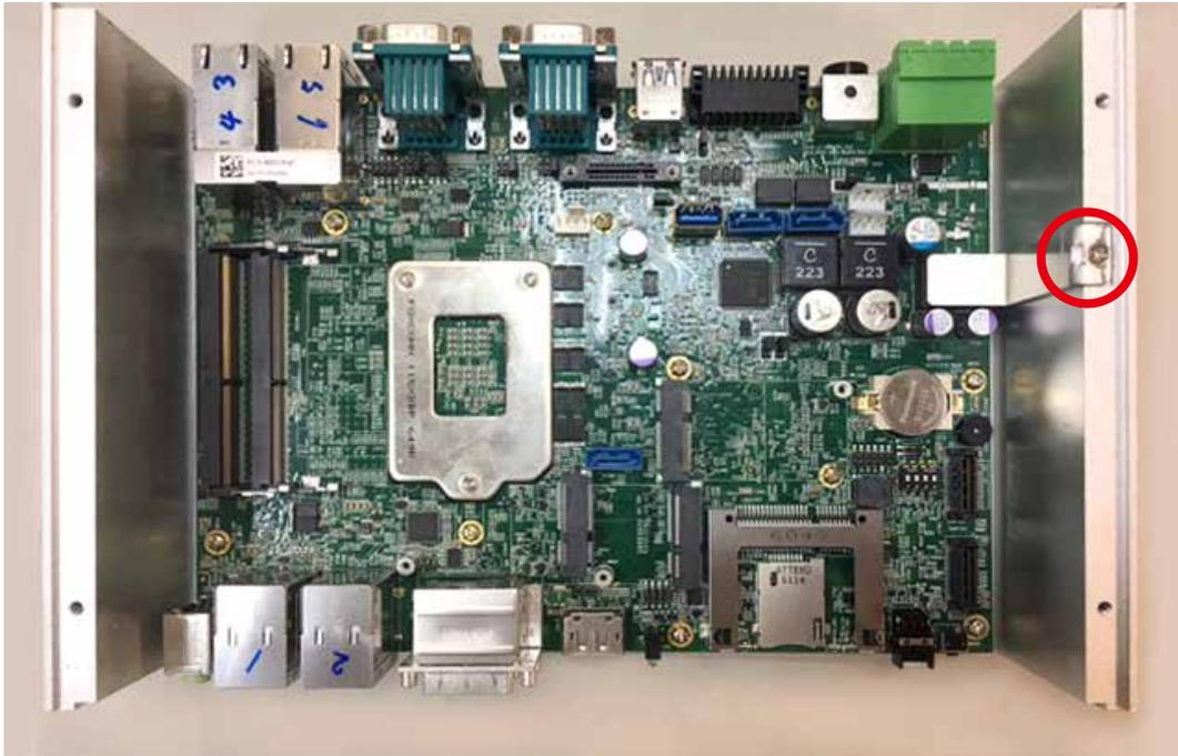
**Step 2** Remove eleven PH-M3 screws and pick up mother board.
