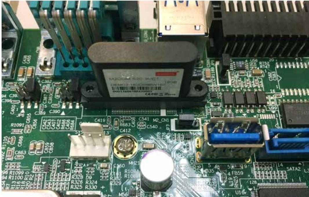
**Step 4** Lock two M2 screws with slot.
