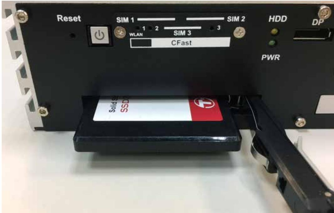
**Step 4** Lock the SSD/HDD tray with key.
